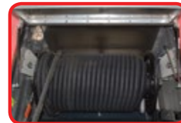
Longer reinforced high pressure hose – 80 meters. Electrically driven reel for automated winding off hose in vertical and horizontal position.
