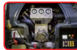
New pump NH-35. Efficient fire suppression with water and foam, working on the normal and two high pressure stages. Control in the compartment or from the driver's cabin. Pump durability allows using even sea water and passing objects up to 8 mm.
